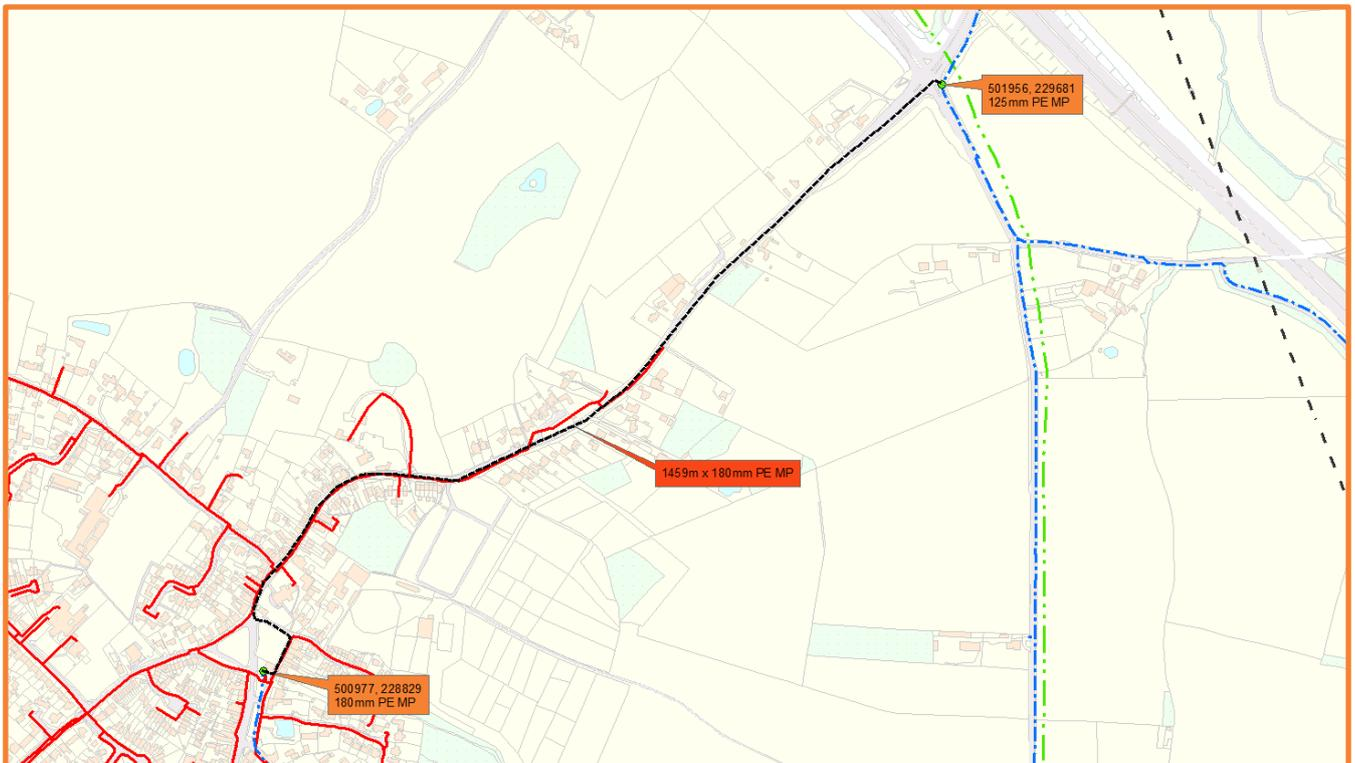
Figure 5 – Route of reinforcement
