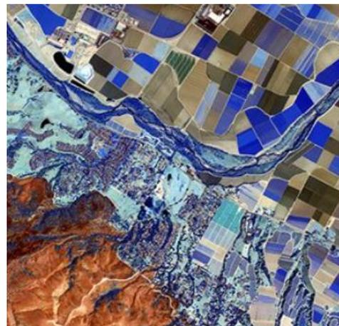
An alternative satellite technology (**SAR imaging**) works in the same way as optical imaging but uses its own 'light source' to emit waves which are reflected from the Earth and detected by the satellite. Water can be easily detected in this imagery including different compositions or levels of ground moisture. This allows algorithms to explicitly detect 'drinking water mixed with soil' from SAR imagery making it very useful for leak detection from water distribution networks.
